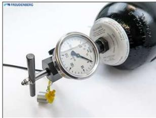
Center the gas valve stem in the locating bore, counter it at the stems key faces and tighten the retaining nut with 50+5 Nm.
