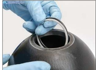
Dismantle the anti-extrusion ring from the valve body, fold it carefully only as far as necessary, and pull it out through the vessel opening.
