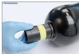
Re-lube the oil-side locating bore. Fold the anti-extrusion ring slightly and insert it through its locating bore into the interior of the vessel as carefully as possible.
