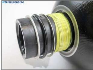
Slide the spacer ring over the fluid port housing and position its centering shoulder in the gap between the housing and the vessel.
