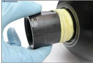
Guide the fluid port housing at its threaded end through the locating bore and position it, i.e. the centering chamfer of the anti-extrusion ring on its counter surface in the vessel.
