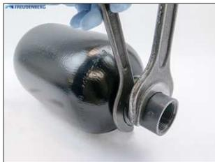
If required, fill the bladder to the set pre-charge pressure.
