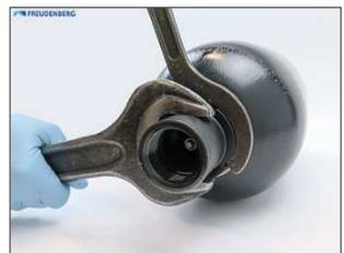
Carefully push the fluid port assembly into the vessel and position it so that the sealing and the anti-extrusions ring can be handled.
